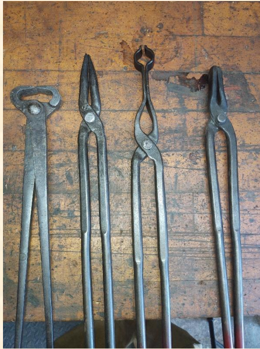
IMAGE: Some tongs from the author's collection. From left to right: nippers, scrolling, pick up, and flat jaw tongs
